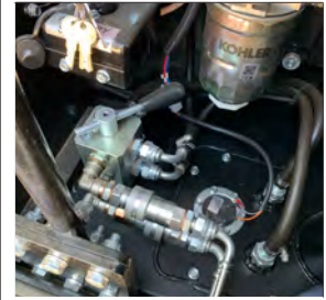
Three Way Fuel Valve For external fuel tank Connection
