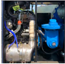
Shaft Drive Vacuum Pump Eliminates issues associated with belt drive versions.
