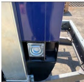
Four Low Level Securing Points To avoid the need to strap over the canopy causing damage
