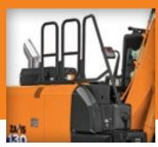
Upperstructure handrails provide added safety when servicing the engine compartment.
